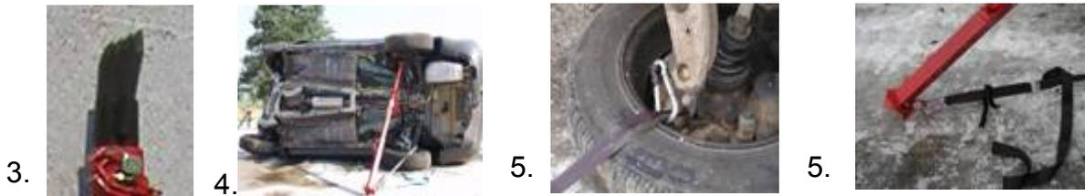
3. Mount the four-pointed tool on the top of the *StabiLift*.
